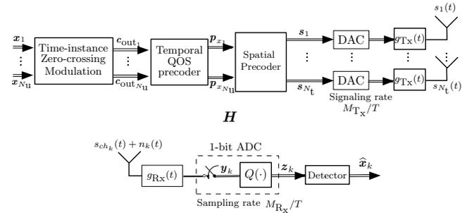
Fig. 1: Multiuser MIMO system model
