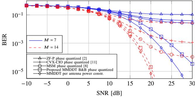
Fig. 3: Uncoded BER versus SNR,  $K = 3$ ,  $\alpha_s = 8$  and  $\alpha_x = 8$
