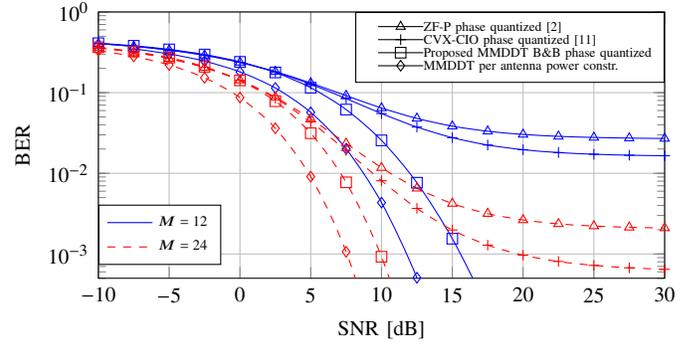
Fig. 4: Uncoded BER versus SNR,  $K = 3$ ,  $\alpha_s = 4$  and  $\alpha_x = 3$
