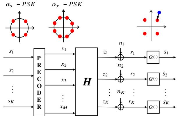
Fig. 1: Multiuser MIMO downlink with phase quantization and hard detection
